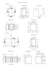
This stainless steel combinable console system, MPCS, has a IP 55/56 protection degree. It includes three interchangeable sections, top, desk and bottom. The system is very flexible and the various possible combinations can meet many design requirements. The ergonomic design of the top and desk units allows for easy installation and access to HMI-equipment, plus increases the mounting space available. This console can be installed in virtually any environment, grade dependent.
